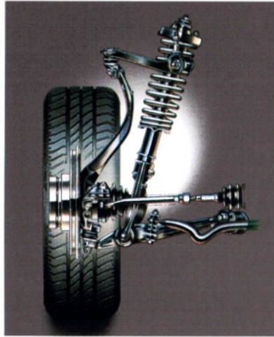
Double wishbone front suspension uses upper and lower arms to precisely control suspension movement for optimum cornering traction.
