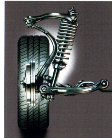
To cancel unwanted rear wheel steering effects when accelerating, braking and cornering, the Accord's double wishbone rear suspension uses toe compensating lower arms.
